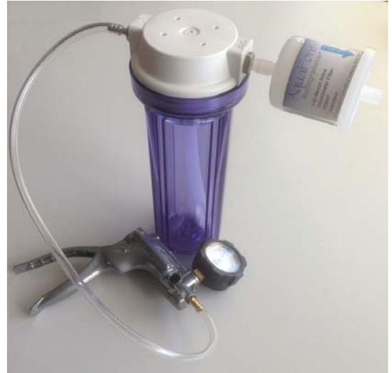
**Like to sample direct from the Bailer?** FTS has modified the BioBailer purging device to make it fit 12 mm ID tubing. Push the tubing over the AquaPore filter\* inlet on one end and over the purge device on the other end and the water will flow out of the bailer directly through the filter. It may have slower flow rates but it works and is low cost.
