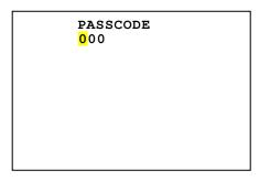
Use the "ARROW" keys to enter the first digit of the passcode, then press the "ENTER" key to proceed to the next digit. Repeat until all three passcode digits are entered.
