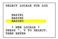
A log locale may be selected by pressing the UP and DOWN keys until the desired locale is highlighted. Pressing the ENTER key will display a Log conformation screen.
