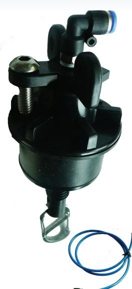
The TriCap-LOG is the perfect choice for use with submersible groundwater level logging devices. It features an elbow fitting which vents the well to the atmosphere, and a unique stainless spring clip for easy logger attachment.
