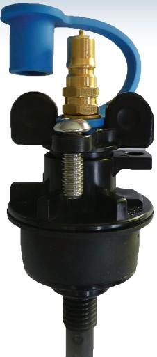
The TriCap-GAS has a quick connect gas fitting and dust cap installed in the top. This enables gas in the well to be withdrawn and sampled with a gas instrument or suitable pump without removing the TriCap.
