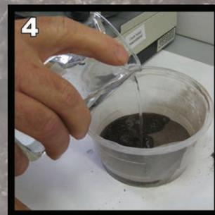
**4.** Weigh out 1 unit soil (100 g is recommended) and put 2 unit (200 g, 2 dl) distilled water to it.
