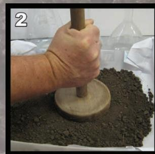
**2.** Shred the dry soil and mix the samples. You will get a homogeneous sample. It mustn't contain rocks or organic residues. Take a sample from this mixture for the measurement.
