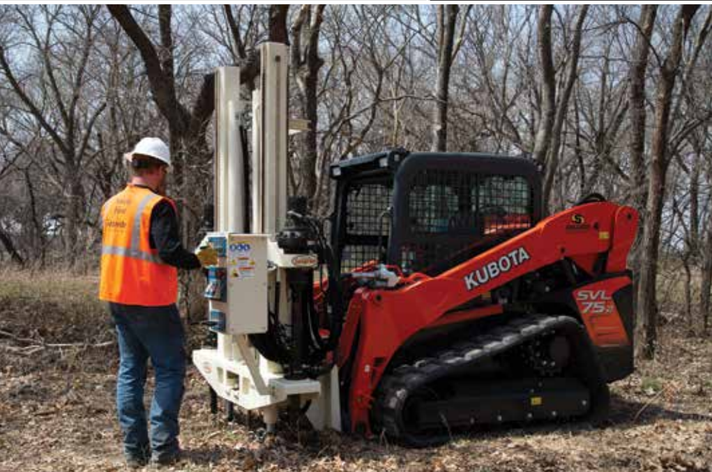
The Geoprobe® 20CPT Press mounted on a skid steer.
