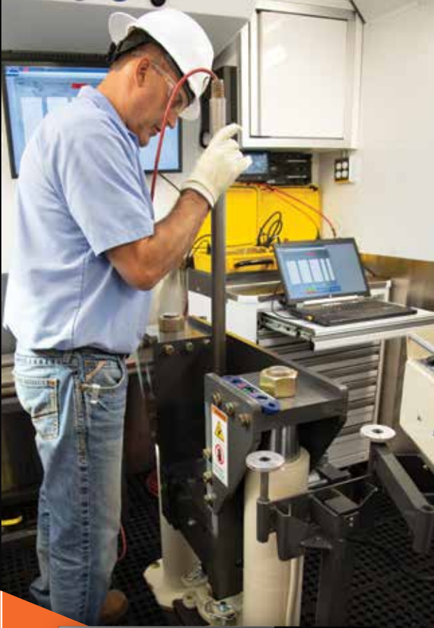
The CPT equipment is placed into the push clamp for testing.
