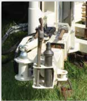
7-in. Breakout Storage Rack Weldment
