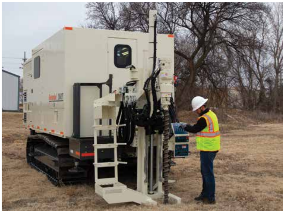
The optional 6712DT mast allows for coring, conventional soil sampling, shallow drilling for soil verification, and pre-drilling.
