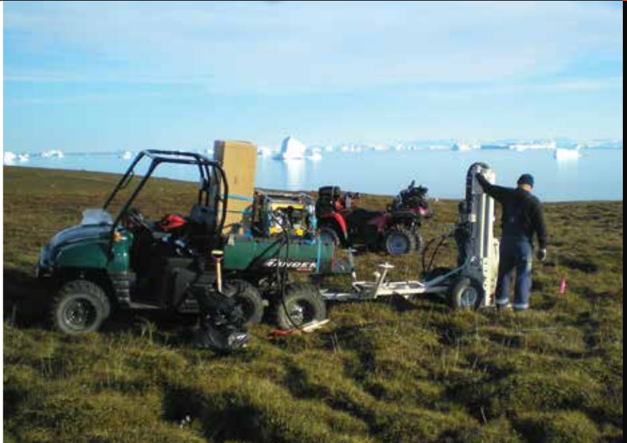
A 540MT is used for geotechnical surveys at a potential mining site in Greenland.
