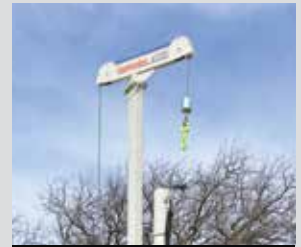
Hydraulic Winch and Mast
